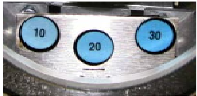
Figure 10. Humidity Indicators (Blue is a Normal Dry Condition)
